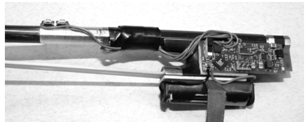
Figure 3. Electronics of the NOTAM bow (total weight ca 25 g including a 12 g AAA battery).
