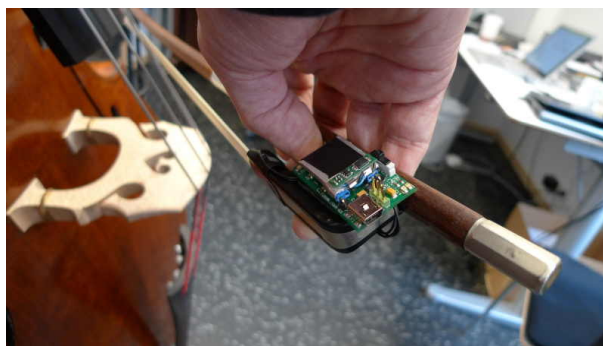
Figure 1. The sensorbow developed at the Norwegian Academy of Music in cooperation with NOTAM, here as a bass bow.
